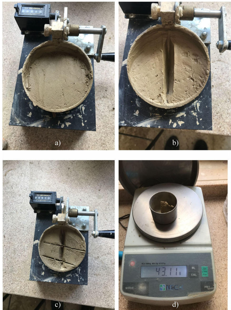
Fig. 5 (a) Placing the sample in the porcelain crucible, (b) Hollowing out, (c) Sampling from the center, (d) Weighing
