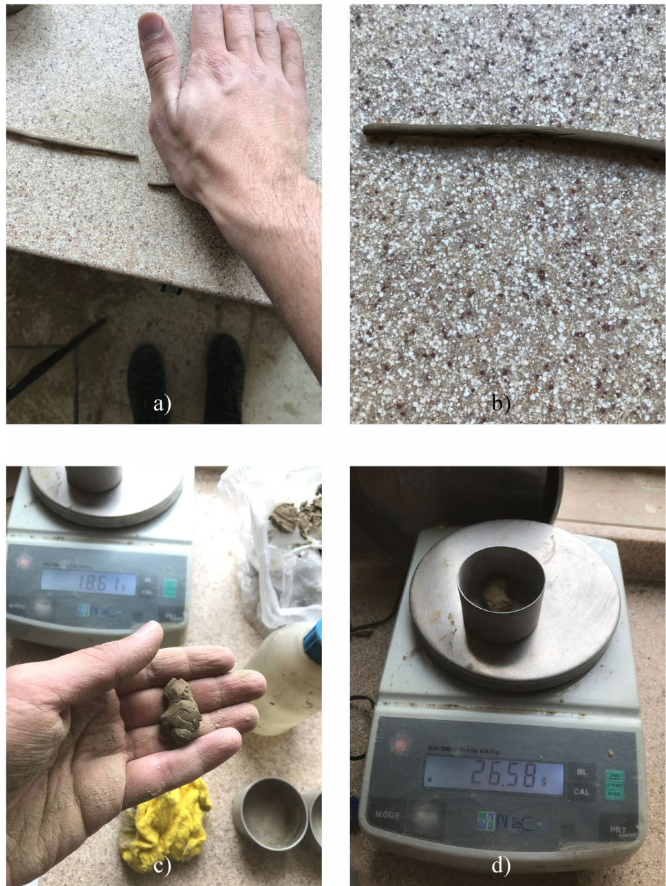
Fig. 6 (a) Thinning the specimen to 3 mm diameter, (b) Cracks are seen, (c) Making the specimen whole, (d) Weighing
