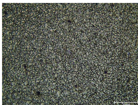
Figure 6. Microstructure images of the cast AZ91/15% SiC/0.8% AlN composite.
