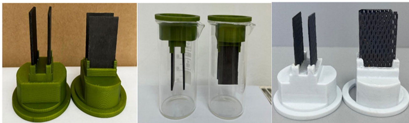
Fig. 1 Graphite (left) and titanium (right) electrode plates with custom 3D-printed PLA holders used in electrolysis experiments. Electrode dimensions: 25 \times 40 mm
