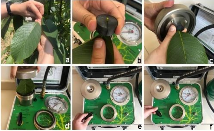
Figure 1. Leaf Water Potential Measurement with Pressure Chamber
