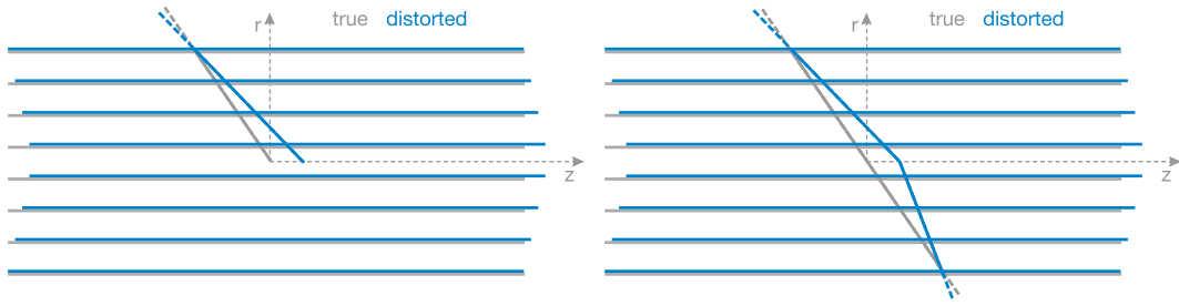
Fig. 5. Diagram demonstrating distortions of the tracker geometry that may not affect the consistency of a reconstructed collision track with the measured hits (left), but introduce a kink when reconstructing the two halves of a cosmic ray muon track (right), leading to an inconsistency. This illustrates the telescope effect from Table 1.
