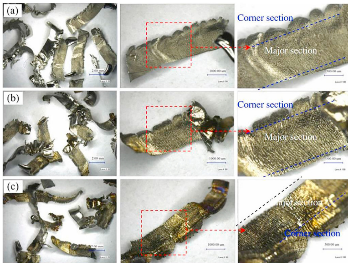
Fig. 3 – Chip morphologies (feed per tooth f_z = 0.06 mm/z, axial depth of cut a_p = 1.5 mm, radial depth of cut a_e = 5 mm). Cutting speeds: (a) v_c = 150 m/min; (b) v_c = 300 m/min; (c) v_c = 450 m/min [66].
