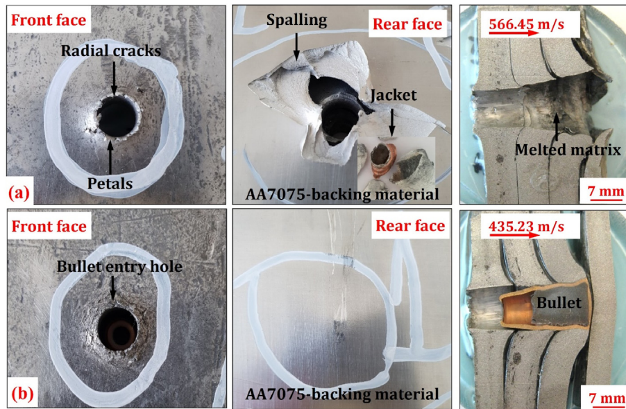
Fig. 16 – Ballistic test results of Al6061/8 wt% Al 2 O 3 reinforced FGMs at a) 566.45 m/s b) 435.23 m/s.
