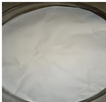
Fig. 3 Photograph of PVDF-HFP nanofiber structure deposited on the surface of the collector plate
